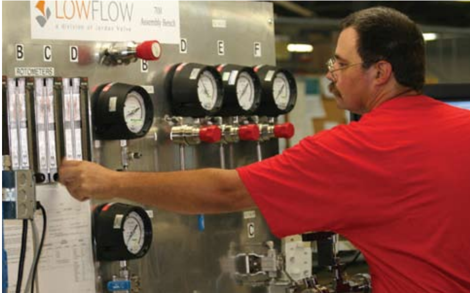
Flow testing with nitrogen
