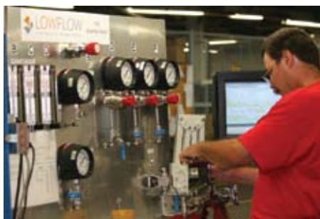
The stem and orifice are installed into a special test fixture
